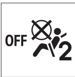
Passenger side SRS airbag OFF indicator light
